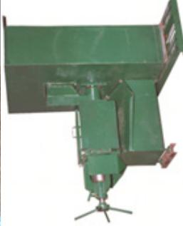
OIL EXPELLER POWER: 8.0HP<br>MOTOR/ENGINE CAPACITY:<br>80KG/HOUR                                                | 6 mill  | SIDO IRINGA |
